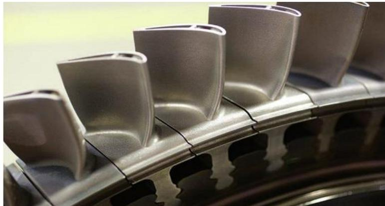
**Fig. 3 Industrial gas turbine printed blades [4]**
