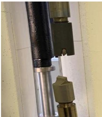
**Fig. 12 Test specimen for fir-tree root after fracture at high temperature**
